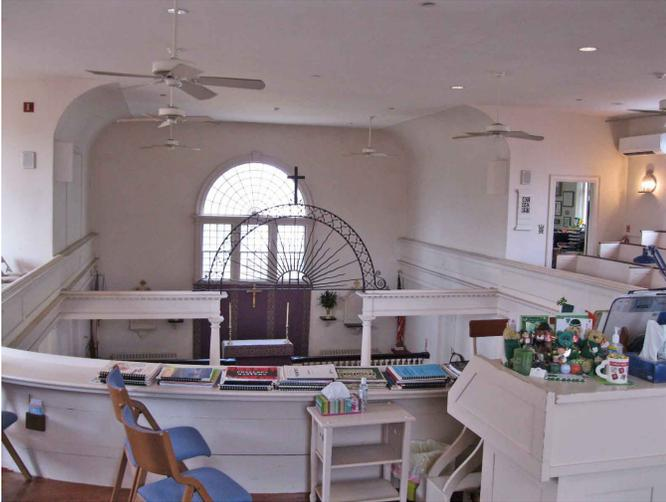
Heat pumps are now being installed in HOWs in the full range of spaces, from offices to meeting rooms and sanctuaries. The photo at left show a wall-mounted mini-split at the upper right. It is one of several serving the space, here in conjunction with fans that move in both directions, thus serving in both winter and summer.
